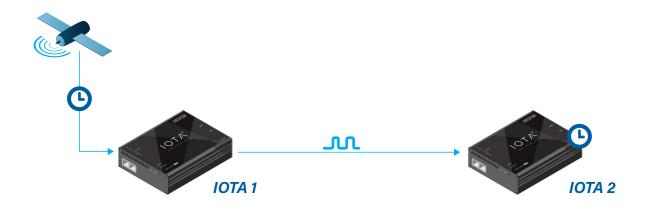
Fig 3. Method 1: relying on 1 GPS signal.
