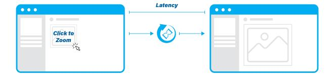
**Fig 1.** In network monitoring, performance can be linked to the concept of latency, referring to the speed of the network or the Remote Response time.
