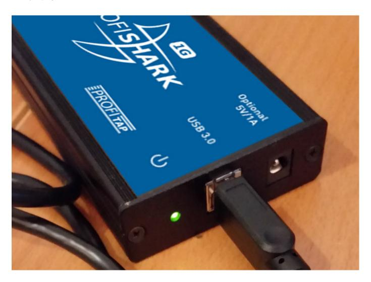
The engineers have thought of that though, and provide an optional 5v connector to power the TAP without being connected to USB – but you need to have an additional power supply for that. At least in my box there wasn't one. It's not really a big thing, but something to consider in data center capture situations – most people do not like link down synchronizations happening too many times in data centers;-)
